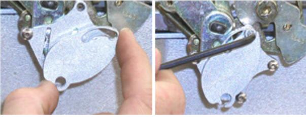
Align the roll pins on the back side of the cam into the slots on the linkage adapter face plate. Once the cam is indexed correctly, install the 8/32" cap screw and tighten using the provided 9/64" Allen wrench. Again be careful not to over tighten this small screw.
