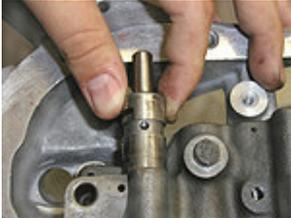
You will then need to remove the TV Plunger and the bushing. To do this, simply pull the TV plunger and bushing out. Now remove the old spring. If the TV plunger and bushing prove difficult, you can make the TV plunger act as a slide hammer by simply pushing it all the way in, release it in such a way as to cause it to "snap" back out, repeat this action as necessary until you get it removed.
