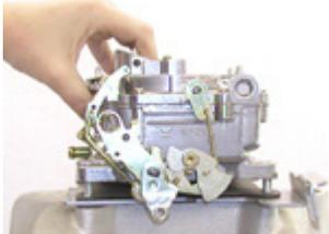
Remove the carburetor and gasket from the manifold. Make sure that the gasket surfaces are clean before you proceed to the next step.
