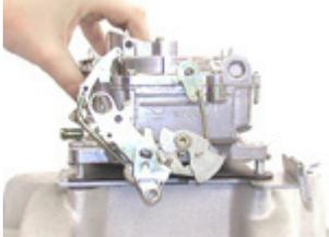
Put your carburetor back on the manifold. Reconnect all the hoses, wires and linkage disconnected when removing the unit. Tighten the hold down nuts evenly using a cross pattern; applying a little more torque each sequence. This procedure will prevent damaging the carburetor.
