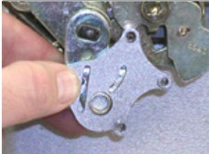
Position the front face plate of the linkage adapter over the linkage as shown in the picture on the left. When correctly positioned, this face plate will index over the extruded (raised area) hole on the linkage. Once indexed over the extruded hole, simply turn the face plate until the four bolt holes line up with the back plate section installed in the previous step.
