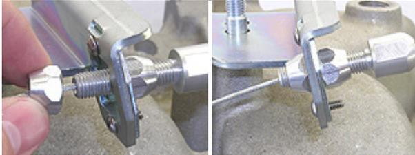
Screw the first adjuster nut back onto the cable adjuster housing. You're now able to make the proper starting set up of the TV system by screwing these nuts along the threaded area of the cable adjuster housing. Moving the position of these two adjuster nuts along the threaded area of the cable adjuster housing relative to the adapter plate will allow you to "preload" a slight pressure boost. Attach the pressure gauge and hose assembly. Refer to Section 4 for pressure gauge installation.
